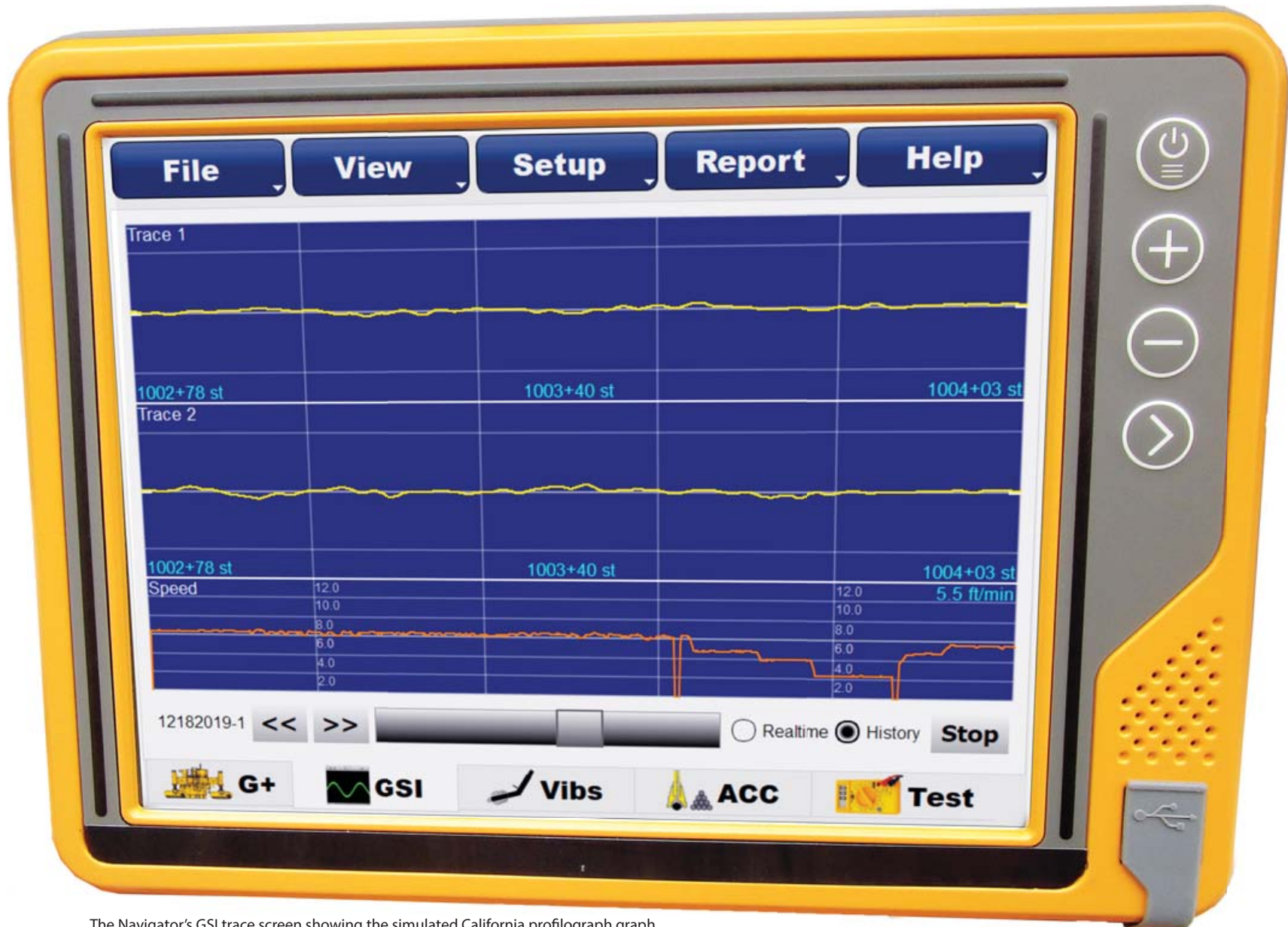
The Navigator's GSI trace screen showing the simulated California profilograph graph.
